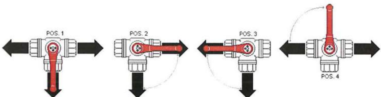
In order to obtain position #3 and #4, remove the lever from the pushrod and replace the lever at 90° (left direction)
